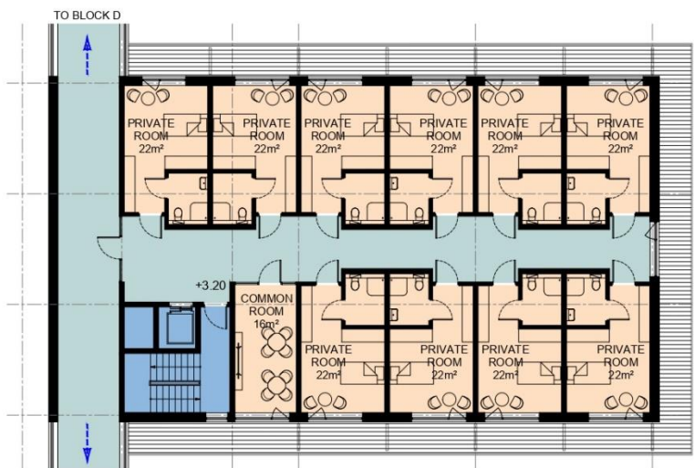
1st. FLOOR PLAN SCALE 1:200 BLOCK C
